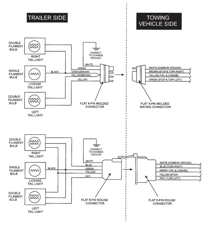
Figure 60. Trailer/Towing Vehicle Wiring Diagram
